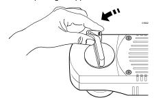
Releasing the lever manually
