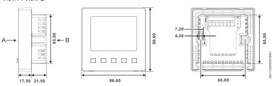
Above are the dimensions for the thermostat and its mounting plate.
