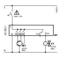
N1 RDF310.2/MM V1 On/off valve AC 230 V M1 3-speed fan
