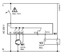
N1 RDF310.2/MM V2 Electromotoric actuator, e.g. SUA21/1 M1 3-speed fan
