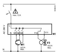
N1 RDF310.2/MM V3 3-wire on/off (SPDT) zone valve M1 3-speed fan
