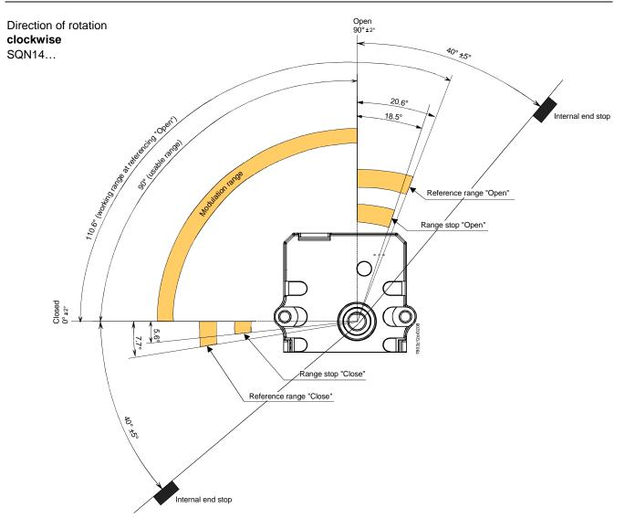
Turning the drive shaft back to the working position If, due to external influences, the drive shaft leaves the working range without automatically returning after resetting the basic unit, it can be cautiously turned back manually. To do this, disconnect power to the plant and drive the actuator cautiously to the beginning of the usable range.
